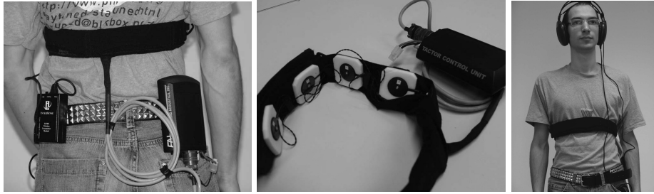
Fig. 1. The waist-belt system consisting of the vibro-tactile belt, the Intersense transceiver, and the belt controller, a detail view of the waist belt, a participant wearing the belt and the headphones in a two-dimensional indoor navigation experiment (from left to right)
